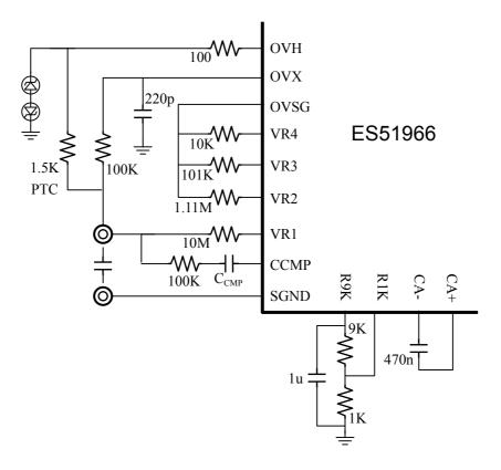
Figure 10.1 Application circuit of capacitance measurement
