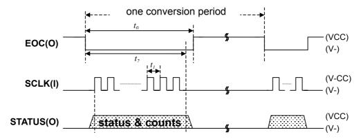
$t_0$  is at least 5ms and  $t_1$  must be  $(32 \sim 512)T$ , where  $T = 0.25 \mu s$ .
