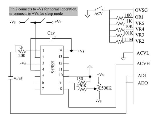
Figure 4.2 AC-to-DC circuit using ES636
