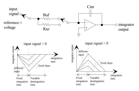
Figure 2.1 the structure of dual-slope integrator and its output waveform.
