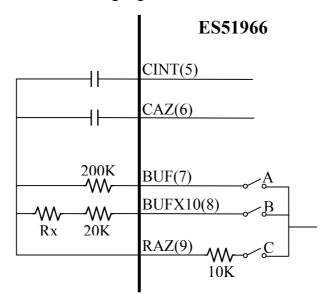
Figure 5.2 Resistor scheme of AZ phase
